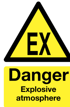
Figure 5 Example of warning sign with supplementary text used at entry points to locations where a potentially explosive atmosphere may exist
